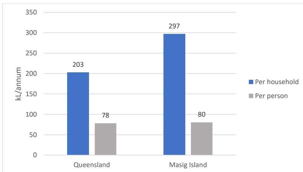
Figure 13: Residential water consumption on Masig Island compared with the Queensland average (2016/17 FY)
